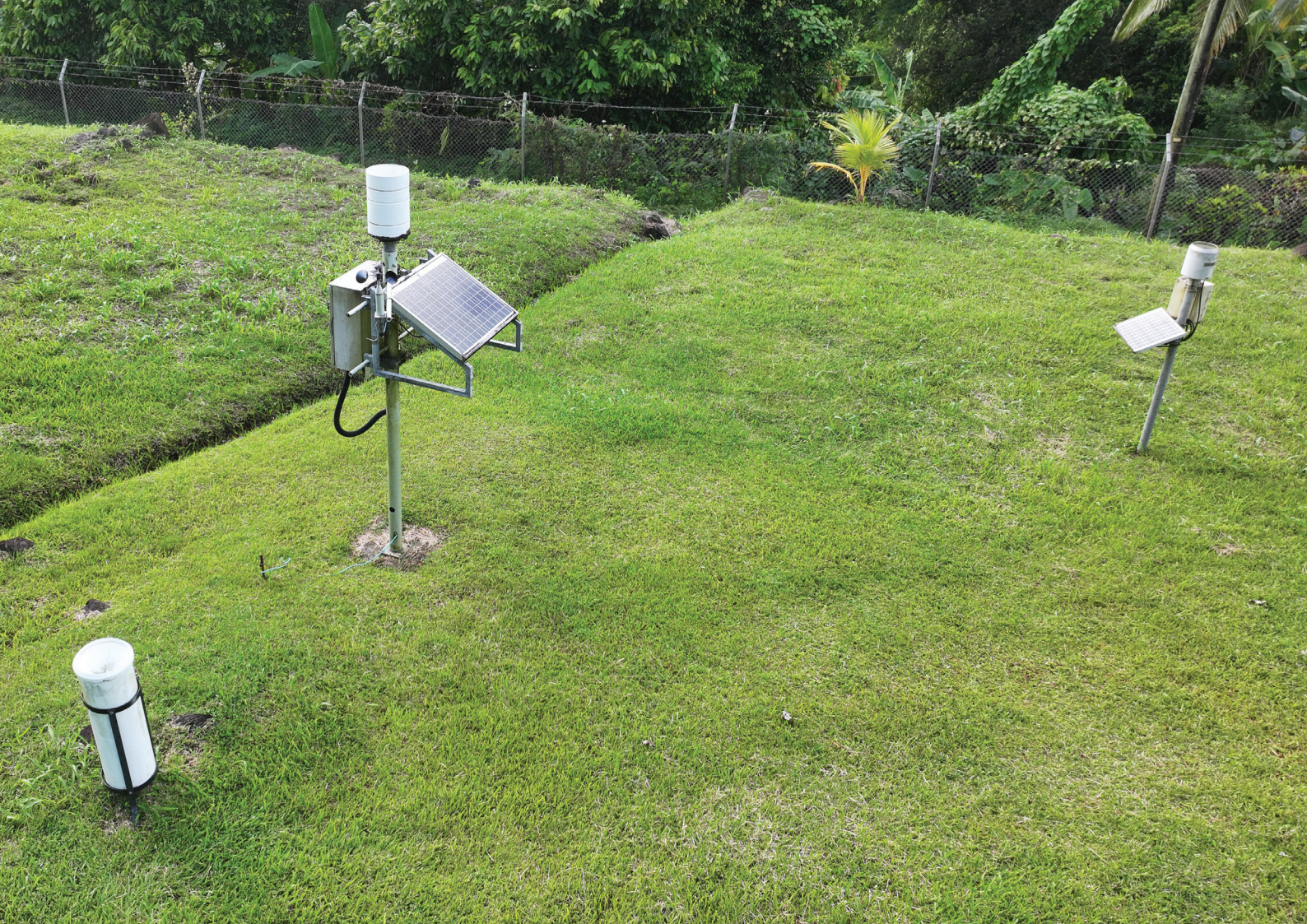
Rain Gauges, at NAWASA Plant in Grand Roy, St. John
